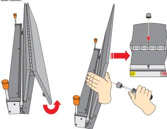
Place the unit in horizontal position on a table or on a proper work surface and set it in a comfortably reachable way. To ensure a correct operation of the unit, the table or surface where you place the unit must be perfectly leveled, easily accessible, not subject to excessive vibrations and at a suitable height (80 - 85 cm [32" - 35"] from the floor level).
